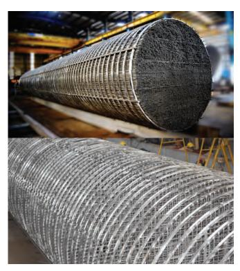
Fig. 3: Tube & Rod Assembly
