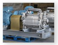
Two-stage Liquid ring vacuum pump
